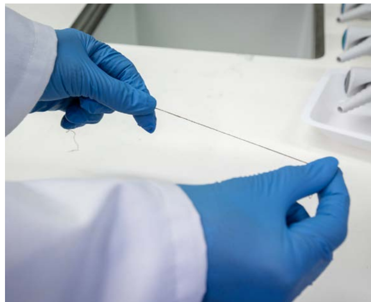
A suture composed of polymers with iodine and nanoparticles (ie, carbon dots) added is currently being studied. Photo courtesy of Shadi Houshyar.
